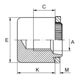
Female thread A = M10Height K = 14.0Min thread length C = 6.0Outer diameter E = 19.0Plate thickness = 1.1 to 1.3Recommended bore diameter for extreme load = 15.0
